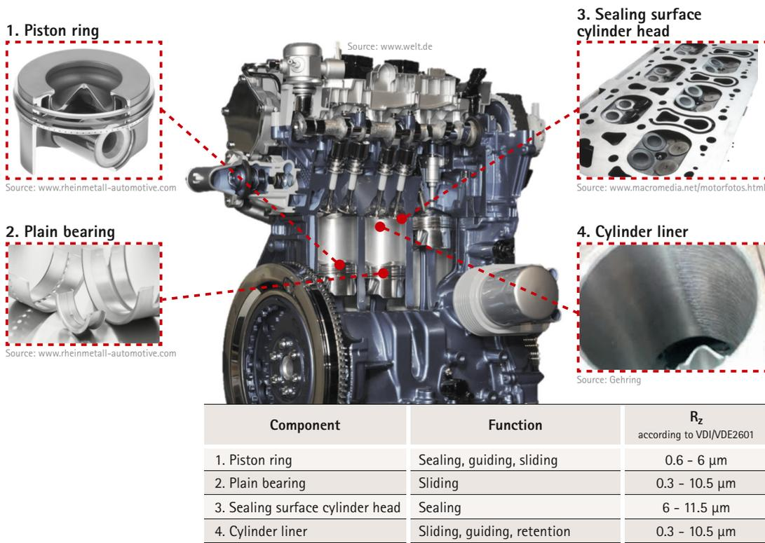
Figure 4: Selected function surfaces based on the example of a large combustion engine
