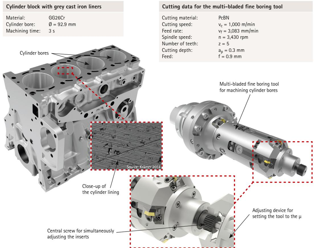
Figure 6: Fine boring cylinder linings on a grey cast iron crankcase with depiction of the tool concept, cutting parameters and a section of the functional surface
