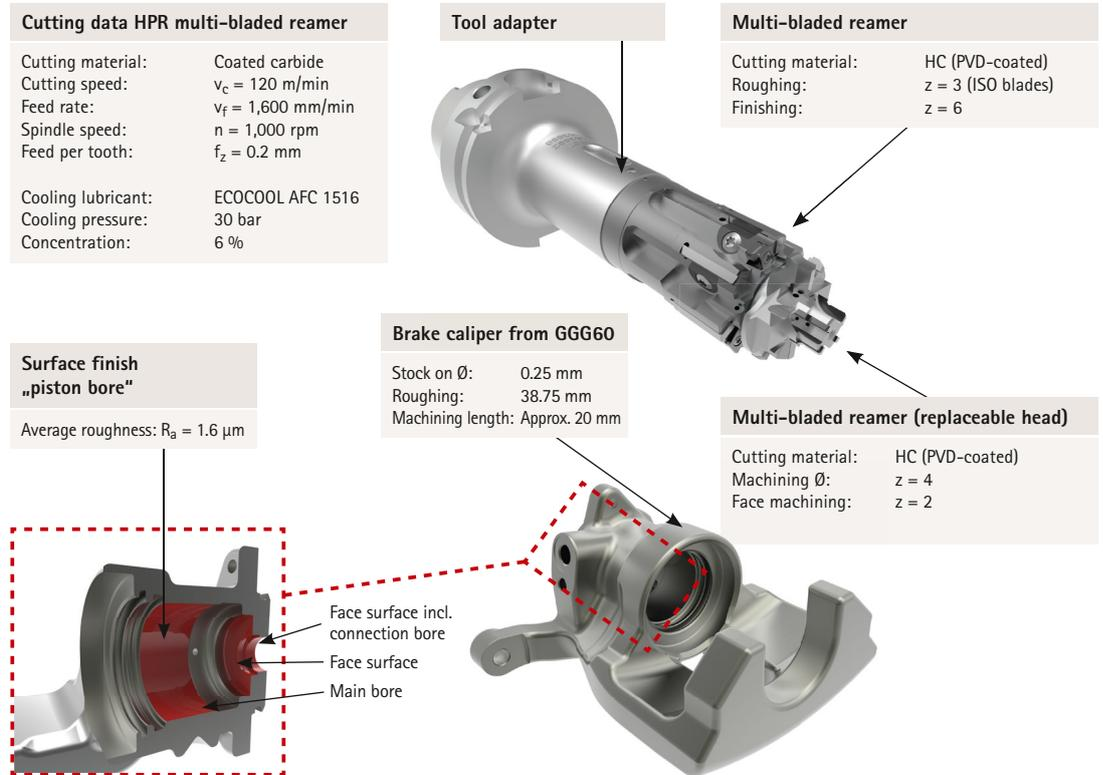
Figure 8: Functional surface machining on a brake calliper made of GGG60 – presentation of tool concept, technology parameters and surface quality achieved
